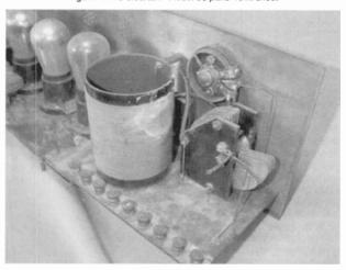
Figure 5. The inside was dirty and the remanants of a dirt dauber's nest can be seen on the side of the tuning coil.
