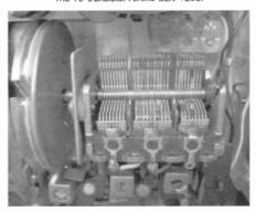
One sign that an RF amplifier is included in an AM radio is to observe that the tuning capacitor has three sections, as in the above picture
