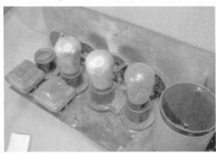
Figure 7. The unrestored inside view showing the loss of nicket place
