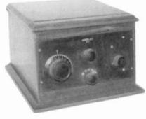
CROSLEY MODEL 51-S-This 2-tube regenerative receiver with binding posts inside is the standard Model 51 in a deluxe cabinet. It was manufactured by the Crosley Radio Corporation of Cincinnati in 1925. (Clark Trissell – Lincoln, NE)
