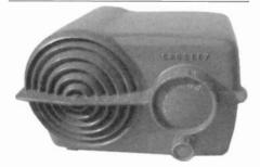
CROSLEY MODEL 11-115U – This maroon, plastic, table radio was manufactured in 1951 by the Crosley Radio Manufacturing Company of Cincinnati, Ohio. Its 5-tube chassis tuned the broadcast band only. The whole 11-series of "Serenader" table radios came in assorted colors. (Dave Crocker – Mashpee, MA)
