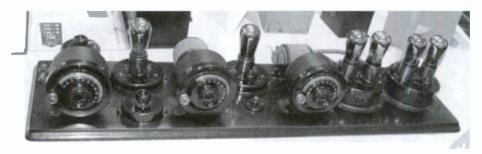
This excellent example of Atwater Kent's top-of-the-line, 6-tube, Model 12 breadboard was Ken Lowther's entry in the old equipment contest.
