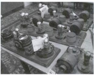
Several Atwater Kent breadboards were included in the sale. The Model 9, the No. 4445, front left, is the early version. It can be identified by the green painted tube unit, battery terminals, and the Type 11 and Coupled Circuit tuners. It sold for \$1,700. The later versions of the Model 9 had an battery cord and brown painted tube units. The Model 9C had tuning capacitors instead of the Type 11 and Coupled Circuit tuners.
