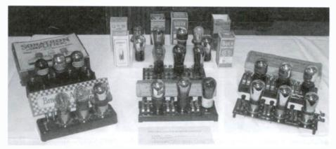
Joe Knight entered this display of 3-tube, resistance coupled, audio amplifiers from 1925 and 1926 in the old equipment contest. The manufacturers, left to right, are Sonatron, Bradley-Amplifier, DeJur, Kelford, Daven, and Muter.
