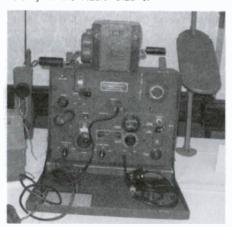
This World War II portable radio station was entered in the old equipment contest. It consists of a BC-654-A transmitter and receiver, and a hand-cranked generator.
