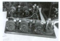
Rear, an even later version of the Model 9C breadboard, the No. 4660, which uses variable capacitor cans instead of adjustable coils. Front, a Model 10C, the No. 4700, which has an additional RF stage.
