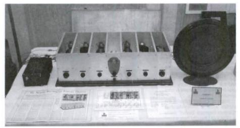
Mike Feldt's 1929, Silver Marshall 710 "Sargent-Rayment Seven," was a blue-ribbon winner in the old equipment contest. Although it looks like an early communications receiver, it covers only the broadcast band. It has four tuned RF stages, with the tuning capacitors all on a single shaft, a detector stage, and two audio stages. The RF circuit, which uses four screen-grid tubes, is claimed to have 10 Kc selectivity. It was available in kit form for \$130 and "built-up" for \$150.
