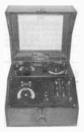
B.T.H. Radiol 1 – This one-tube crystal set was manufactured in 1923 by the British Thompson-Houston Co., Ltd., of Coventry, England. It is stamped "Wireless H.F.-Valve Receiver." It uses a double crystal detector under a transparent holder with two adjustable knobs. The tube is mounted inside under the panel. (Jim Taylor – Winton, Boumemouth, England)
