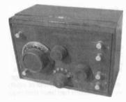
CROSLEY MODEL 50 – This 1-tube regenerative receiver was manufactured in 1924 by the Crosley Company of Cincinnati, Ohio. Its regeneration was achieved by adjusting two spider-web coils with the knob just above the tap-switch on the panel. (Dave Crocker – Mashpee, MA)
