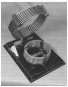
Some may wonder what this strange apparatus is — it is an oscillation coil made by Murdock for use in a spark transmitter. It sold for \$275.
