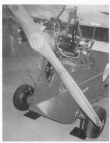
Figure 2. A frontal view of the Flea showing just how close the airplane's engine was to the pilot. There is a flexible hose coming down from the upper wing, which indicates that the gas tank was in the wing. The engine's two exhausts would flow just above the head of the pilot. This was flying in the rough!
