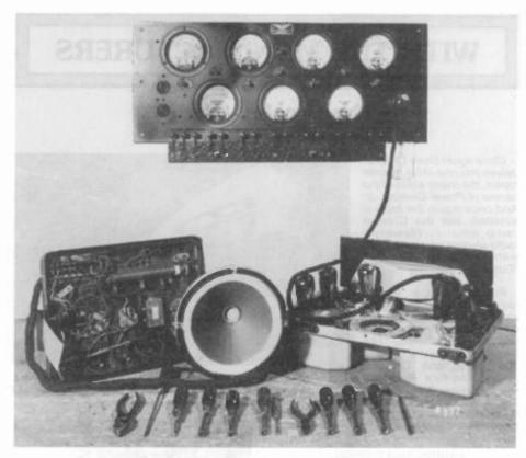
Figure 2. A Jewel radio set analyzer plugged into a Victor Model 45 chassis.
