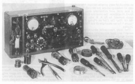
Figure 3. A rare R-K Model V-7 radio test set.
