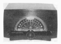
GENERAL ELECTRIC MODEL 409 – This AC-DC table radio in a plastic case was manufactured in 1952 by GE. It operates on the following seven tubes: (3) Type 12BA6, (1) Type 12AT7, (1) Type 12AV6, (1) Type 35Z5, and (1) Type 19T8. It tunes with two thumbwheel knobs on either side of the front plastic extension. (Clark Trissell – Lincoln, NE)
