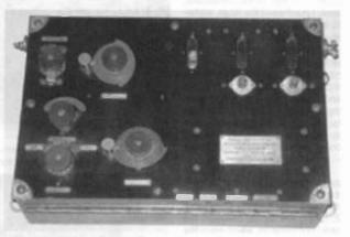
Figure 9. The Western Electric SCR-75 radio aircraft receiver.
