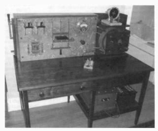
Figure 1. Clapp-Eastham 1-Kilowatt Spark Transmitter.
