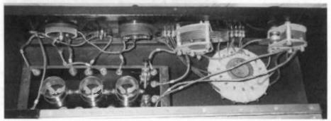
Figure 3. The components inside the set can be seen here. The 3-tube unit on the left actually is a sealed module and weighs about seven pounds! The crystal detector also is mounted on this unit.
