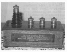
Figure 4. Wireless Specialty Apparatus (W.S.A.) Eaton oscillator.
