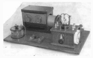
Figure 5. A Spherical Audion breadboard radio.
