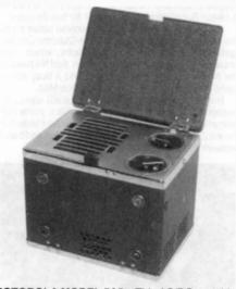
MOTOROLA MODEL 5A5 – This AC/DC portable was manufactured in 1946 by the Galvin Mfg. Company of Chicago. The flip-top is the on/off switch. It operates on one each of the following tube types: 1R5, 155, 1T4, 3S4, and 117Z3. (Clark Trissell – Lincoln, NE)
