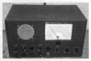
Figure 1. The metal Coast Guard communications receiver Model R-138 with many knobs and a large dial.
