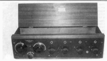
CROSLEY MODEL XJ – Sold by the Crosley Radio Co. of Cincinnati, Ohio, in 1923, this 4-tube battery receiver uses all Type 01-A tubes. It tunes using two "Book Type" tuning condensers made famous by Crosley. (Clark Trissell – Lincoln, NE)
