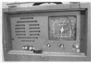
Figure 7. Seen at the lower front, an added microswitch that switched off the filament battery when the front cover was closed.
