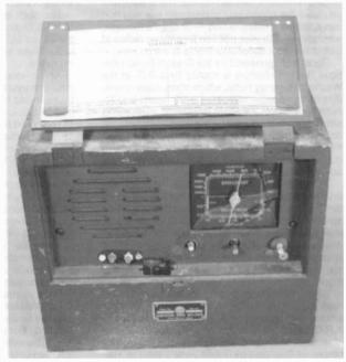
Figure 1. The Templeton BP2-A5 as found and described as "junk" by one viewer and "cute" by another. The raised cover shows a station log card.
