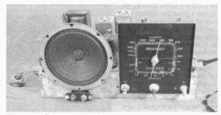
Figure 10. The chassis with several things to repair, but with a speaker cone in remarkably good condition.
