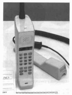
An early "cell phone" by Motorola, the "TacTek." Selling for \$3,995 in 1983, it weighed 16 oz. It was based on the original Motorola "DynaTac," developed in 1973, which weighed 3 lbs. It contained 30 circuit boards, and you could talk for up to 35 minutes on a charge. DynaTac stood for "Dynamic adaptive Total area coverage."
