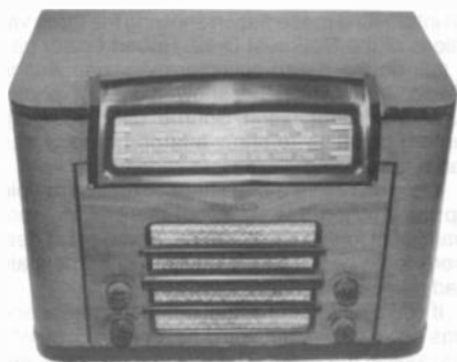
PHILCO MODEL 41-240T – Made by Philco in 1941, this wood table radio operates on seven tubes and tunes in the broadcast and shortwave bands. ( Clark Trissell – Lincoln, NE )
