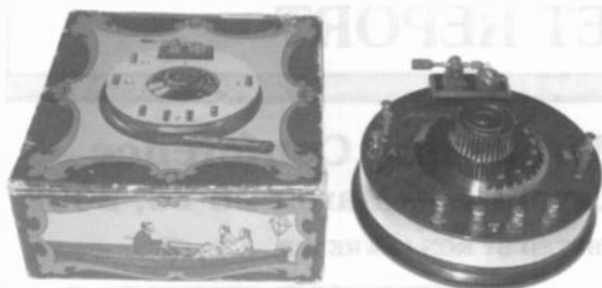
"MAGICUS" CRYSTAL SET – The "Magicus" crystal set, right, was built by Optik-Aktiengesellschaft E.A. Juch in Berlin in 1925. It still has its original plug-in detector and the impressive original carton, left. ( Erwin Macho – Vienna, Austria )
