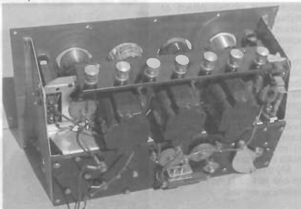
Figure 5. A rear view of the chassis of the later version of the Kennedy Model VI. Note that the seven binding posts are mounted atop the chassis.
