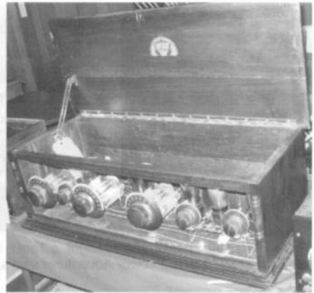
This Supertone glass-front, 5-tube battery set from the Cleveland Auto Accessory Co. sold for $350.
