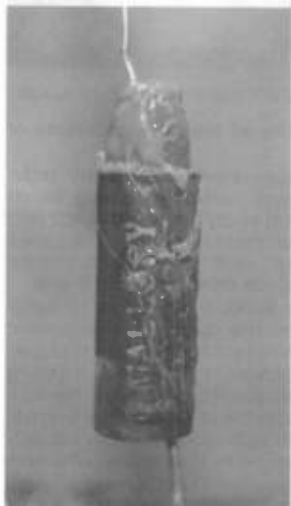
Figure 3. As the wax melts, the sleeve of the capacitor will slide downward.
