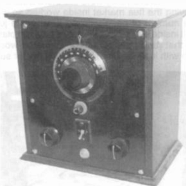
HOME-BREW RECEIVER – This home-built receiver has a one-dial tuner and operates on three tubes: two Type 01-As and one Type 199. The cabinet is also home-built. ( Wally Worth – Wollaston, MA )
