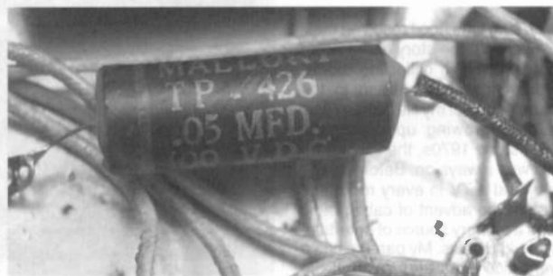
Figure 13. The rebuilt capacitor mounted in place of the failed capacitor. Compare to Figure 1.
