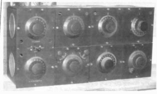
This six-unit Amrad receiver is a rare item. It includes four of the square, single-unit sized pieces, and two rare double-sized units. On the left end is the vertical 3071 2-stage RF amplifier, and on the upper right is the 2776 2-stage audio amplifier. Unfortunately, all of the unit identification tags were missing.
