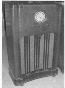
Above, to the right, and on the opposite page, are photos of the Airline 6F which sold for \$1,500. Although this 16-tube, 4-band console is simple in appearance from the front, the rear view reveals two Scott-like quality chassis and two massive speakers.
