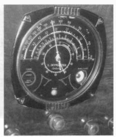
On the left is the elusive Imperial SkyMaster console, and above is a close-up of its dial face. Note the tuning eye tube mounted on the right side of the dial face. This console radio was in very good condition and sold for \$150.
