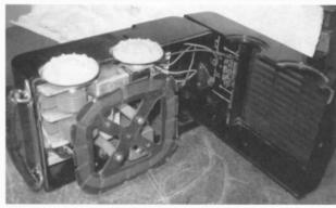
Figure 3. The KG-80 Candid shown open so the "Air Magnet" loop antenna can be seen.
