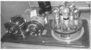
This Atwater Kent Model 8 breadboard sold for \$900. The 5-tube unit on the right (a 2-stage RF amplifier, a detector, and a 2-stage audio amplifier) is included also on the Model 5 breadboard.
