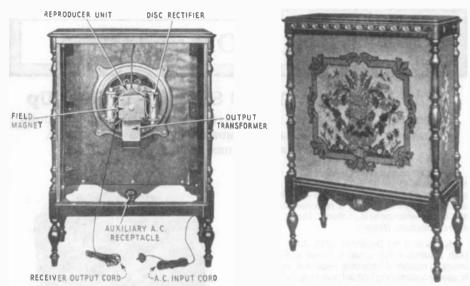
Figure 2. Two images of the Radiola 106 speaker from the "RCA Victor Service Notes for 1923-1928."
