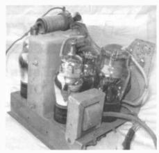
Figure 3. The chassis of the Halson NS-40.
