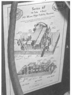
"All-Wave High Fidelity Receiver" claims the paper tag inside the cabinet of the Airline 6F. It also points out all of the vacuum tubes and their functions.
