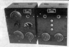
This Campbell Model D detector and Model A2 2-stage amplifier, was a contest entry by Merrill Bancroft. The Campbell Company was known for its medical electric apparatus.
