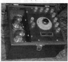
Seen in the flea market, this AeroFone 2-tube amplifier was manufactured by the Prometheus Electric Co., New York. It was designed to be used with the Aeriola Sr. receiver as shown below. The literature with the amplifier claimed that "... it will give results that are almost unbelievable. It will amplify the volume... to such an extent that a loud speaker can be operated."
