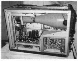
Figure 4. A open left side view showing more tubes. The plug-in is inserted showing the inside wiring.
