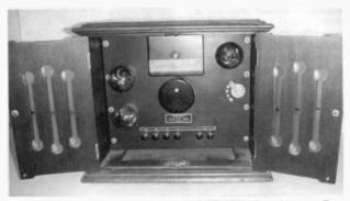
From Western Electric, a Model 14A amplifier/speaker with three Type VT-1 tubes sold for \$600. The horn and grille are on the other side.
