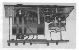
Figure 3. An interior view of Richard Foster's restored set showing the heavy spiral pigtail connections kept from tangling by metal disks on either side.
