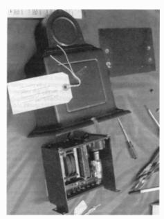
This partially disassembled view of the Western Electric Model 7A microphone shows the amplifier section.
