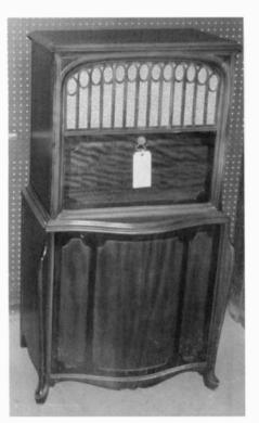
An RCA Radiola Super VIII, ca 1924, in its impressive cabinet. This battery-operated radio sold for \$200.
