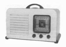
PHILCO MODEL 40-120 – Manufactured in 1940 by the Philco Corporation of Philadelphia, the Model 40-120 has a wooden, painted vivory cabinet. It uses one each of the following tube types: 7C7, 7A8, 7B7, 7C6, 35A5, and 35Z3. It tunes the broadcast and the police bands. (Clark Trissell – Lincoln, NB)
