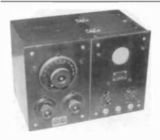
WESTINGHOUSE MODEL RC – This 3-tube receiver was manufactured in 1921 by Westinghouse Electric Manufacturing Co. of East Pittsburgh, Pennsylvania. The Model RC is a combination of the Type RA shortwave tuner and the Type DA detector/amplifier in one cabinet. The earlier 2-cabinet model was called the Type RA-DA. (Clark Trissell – Lincoln, NB)
