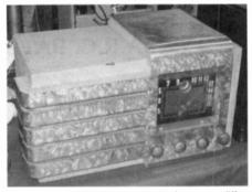
A DeForest Radio Institute radio in a very different cabinet style. Its wood cabinet is flock-covered with a decorative metal facing. It tunes the BC band and features a tuning eye tube. It sold for \$150.
