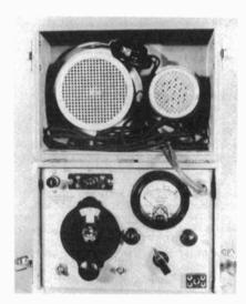
Figure 2. The Type SPF or "Semiportable Fone," 21/4-watt, AM/CW transmitter, powered by dry batteries. (From "Radio for the Fireline")
