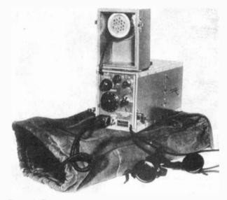
Figure 1. The Type PF or "Portable Fone," a 21/4-watt, AM/CW transmitter, powered by dry batteries. (From "Radio for the Fireline")
