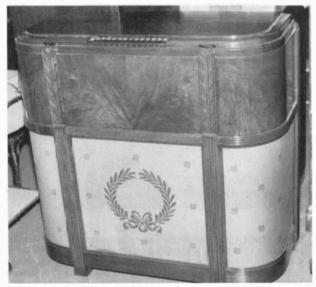
The General Electric Model 695 is an unusual radio. The push buttons operate electric motor-driven controls. It brought only \$50 in the auction.
