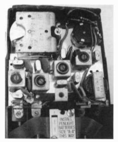
Figure 2. A example of the hand-wired chassis in the early Zenith 500 models.
