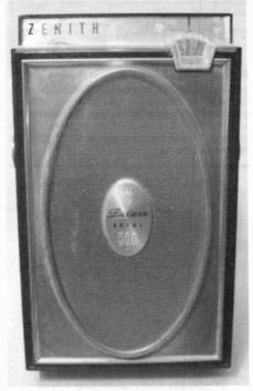
Figure 8. In 1961, Zenith produced its final version, the redesigned 500H with its oval speaker.
