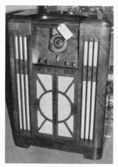
Philco's Model 38-690 is a fine example of highend radios. A 20-tube set, it tunes the broadcast and four shortwave bands. The speaker system consists of a woofer, two tweeters, and resonators. The cabinet features a roll-top door that pulls down to cover the dial and controls. The set was the auction's top-dollar item and brought \$2,100.
