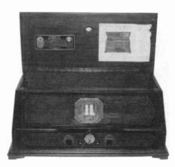
RCA RADIOLA 25 – This 6-tube battery set was manufactured in 1925 by the Radio Corp. of America (RCA). It operates on five Type 199 tubes, and one Type 120 tube for output. It tunes with two thumbwheel dials in the brass escutcheon. The hole in the top lid is for a rotating loop antenna. (Clark Trissell – Lincoln, NE)
