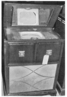
Like the prewar RCA models, this Sparton TV uses a mirror-top to view the vertically-mounted picture tube. The auction price was \$65.
