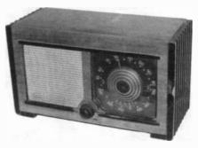
ZENITH MODEL 5D027 – Manufactured in 1942, this 5-tube receiver has an AC/DC circuit and tunes the broadcast band only. Tubes used in the circuit are one each of the following types: 3525, 50L6, 12SO7, 12SK7, and 12SA7. (*Clark Trissell – Lincoln, NE*)
