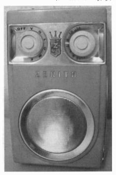
Figure 4. In 1957, Zenith switched from handwiring to printed circuit board construction on this 500B series with its white station indicator on the tuning knob collar.
