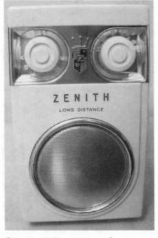
Figure 5. In 1957, a wideband RF amplifier was added to the 500D, making it an 8-transistor radio. It was labeled a "Long Distance" radio.
