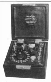
PARAGON MODEL DX-1 – This crystal set, ca 1924, is housed in a black leatherette case that measures 5%" x 3%". It has a push button and a buzzer to test the best spot on the galena detector. (Wally Worth – Wollaston, MA)
