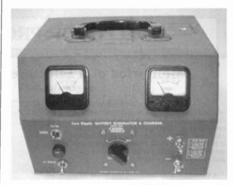
Figure 3: This ratty looking example of an EICO Model 1060 provides 0-8 VDC at 10A continuous or 0-16 VDC at 6A continuous using a transformer with a sliding tap on each of its dual secondaries, and a rectifier with plates the size of a slice of bread. The "Low Ripple" designation on the front panel derives from the Model 1060's extra L-C filter section, not provided in the standard model, the 1050.
