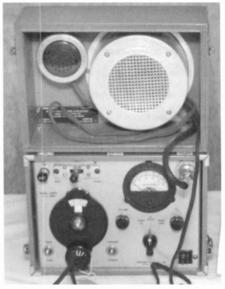
Another Forest Service set appeared in the A.R.C. report for the August 2007 ARCI meet. Manufactured by the Spokane Radio Company, this 1930s 2-way radio, also a Model SPF, operated on 3.2 MHz. In a carrying bag with batteries, it weighed 20 pounds and had a transmitter output of several watts. A five-tube receiver is also included in the cabinet along with the speaker in the lid.
