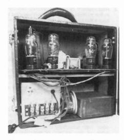
Figure 2. An interior view of the Tom Thumb portable after repairs were made. The battery eliminator is located on the bottom shelf at left. The built-in speaker is at right.
