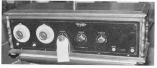
A Hy-Power Super from Victoreen Radio Company. This 2-dialer superhet has three rheostats to control filament voltages.
