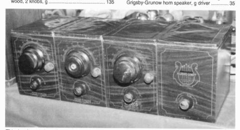
This 4-unit set is in uniform cabinets, but sports three different labels. The left two cabinets are marked "George W. Walker Veri-Unit" and appear to be tuned RF stages. (George Walker is credited as the manufacturer of Victoreen radios.) The third from the left cabinet is marked CARCO, mfg. by Carter Manufacturing Co., East Cleveland, Ohio, and probably is a detector stage. The right cabinet is labeled Audio Unit, The Carter Mfg. Co., Cleveland Ohio. The 4-cabinet combination sold for \$250.
