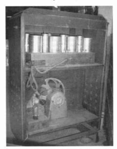
A rear view of the Scott Allwave 15, the two chassis, and the hefty speaker.
