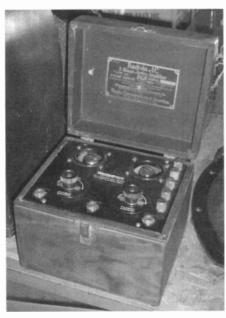
Another early piece — a Radiola AC, 2-tube, audio amplifier, built for RCA by Westinghouse. Complete with tubes, it sold for \$210.
