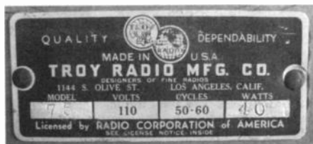
Figure 2. On the rear of the Troy is the nameplate showing the model number "75" and the watts as "40." (Note: These areas on the nameplate have been enhanced so these numbers can be seen more clearly.)
