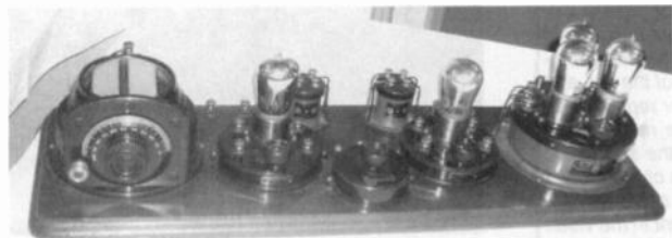
Merrill Bancroft entered this Atwater Kent 4066 breadboard in the old equipment contest. It was Atwater Kent's first 5-tube radio.
