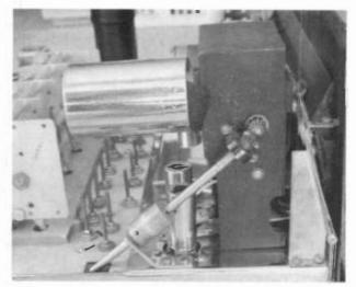
Figure 4. This close-up shows the bandswitch motor, gears, and driveshaft that make up the bandswitching mechanism.
