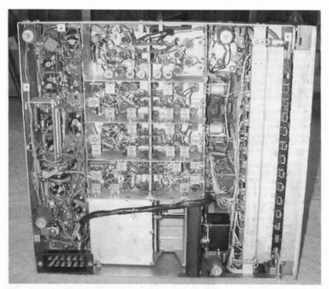
Figure 7. The bottom shield has been removed to show the complexity and component density of the tuner chassis. Maintainability was not high on the designer's list of features.
