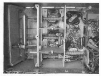
Figure 5. The FM front end employed permeability tuning and a rugged cast aluminum housing.
