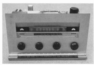
Figure 2. This front view of the receiver shows its clean lines and symmetrical layout. The front panel was designed by John Vassos. The meters indicate signal strength and FM station centering. Audio bandwidth is graphically indicated on the white line below the bass and treble thumbwheels below the meters.
