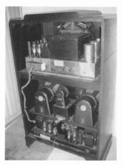
A rear view of the Zenith Stratosphere shows a complete set of chassis and speakers.
