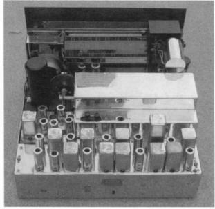
Figure 3. A rear view of the tuner chassis with the bandswitch tuning mechanism at the top left of the photo, the rotating dial scales top center, and the tube layout at the bottom.
