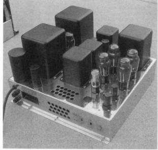
Figure 12. This view of the power supply/power amplifier chassis shows plenty of iron on a chrome-plated chassis. Four Type 6L6G tubes are used in push-pull parallel.
