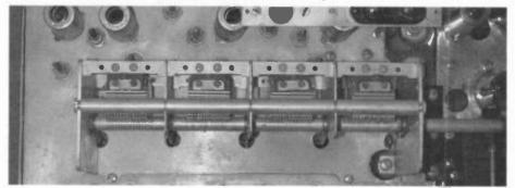
Figure 6. In this view, the cover has been removed to show the 4-gang tuning capacitor used in the AM section.
