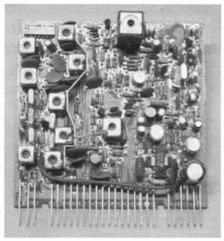
Figure 3. The IF board that was identified as the scurce of the oscillation problem.
