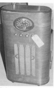
This Golden Tone farm radio operated from 6VDC, tuned the BC and 1 SW band, and featured a tuning eye tube. It sold for \$175.
