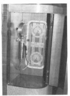
A detailed view of the radio's built-in PA system controls and microphone, an unusual feature even in a high-end set.
