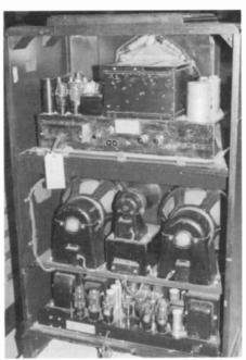
One look at a rear view of the 25-tube Stratosphere and the word "massive" springs to mind. Note the three speakers and heavy-duty amplifier/power supply.
