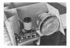
Figure 9. A closeup of the 1st RF stage showing the tuning capacitor. drum dial, plug-in coil and a knife switch which selects the antenna length.
