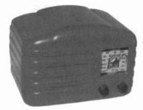
ARVIN MODEL 522 – This 5-tube radio, which is housed in a metal cabinet, was manufactured in 1941 by Noblitt-Sparks Industries of Columbus, Ohio. It uses the following tube complement: one each of Types 12SA7, 12SK7, 12SQ7, 50L6, and 35Z5. (Clark Thissell – Lincoln, NE)
