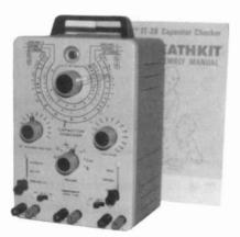
HEATHKIT MODEL IT-28 – This kit-built capacitor checker was offered by the Heathkit Company in the 1960s. (Clark Thissell – Lincoln, NE)
