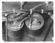
Figure 17. The meter scaling resistors are wirewound on bobbins.
