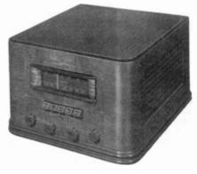
Figure 1. Crosley recommended the use of its Model 1758A high fidelity, 2-band radio to feed its facsimile printer. The radio tuned the BC band and 24 to 47 MHz band. It featured an amplified AVC circuit to control the radio's output level to the printer.
