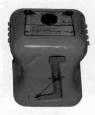
KINGSTON EMERGENCY RADIO — This bright yellow set was used as an emergency lifeboat radio during World War II. It was built by the Kingston Radio Co. of Kokomo, Indiana, which began making farm radios as far back as 1934. Its concave sides were for the operator's knees while he was cranking it for power. The crank fit into the odd shaped recess on the front. (Clark Thissell — Lincoln, NE)
