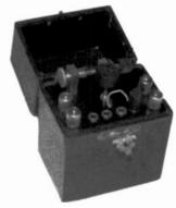
"LILIPUT" CRYSTAL SET – "Liiput" was offered in the radio catalog of Vienna Radio dealer Max Böhnel in 1927. It is a very small, impressive Austrian crystal set with variometer tuning and built-in crystal detector. (Erwin Macho – Vienna, Austria)
