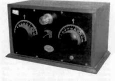
HARKNESS RECEIVER OF 1925 – This 2-tube receiver operates on a crystal reflex circuit. The fixed type crystal detector is mounted at the top center of the panel with a glass dome to protect it. (Wally Worth – Wollaston, MA)
