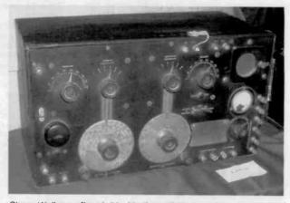
Steve Wallace offered this Medium Wave Receiver, in excellent condition, for \$5,500. The label says that the set was made for the Navy by the American Radio and Research Corp. in 1920 and that its tuning range was 250-7500 M.
