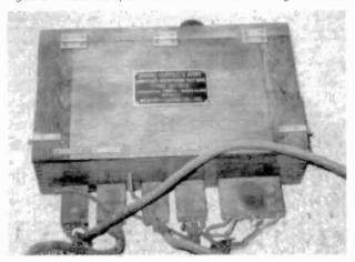
Figure 3. A Type BC-10-A Aircraft Interphone box used to switch between intercom and transmit.
