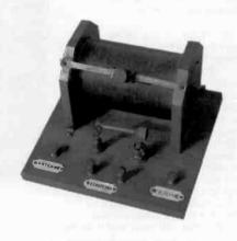
NORMANDIE CRYSTAL SET — This Frenchmade crystal set has a slide tuner and unique detector. The binding post nameplates are ivory, and the coil is made of red enamel wire. The base measures 6" x 6" and the set stands 4" tall. (David Pope — Plymouth, MA)
