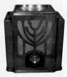
Figure 1. A Remler Model 88, a hi-fi, 10-tube radio from 1935. It featured a 2-way speaker system and a 15-watt, push-pull output stage using Type 2A3 tubes.
