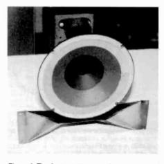
Figure 2. The 2-way system speaker system used in the Remler 88. The woofer is a 6-inch, highcompliance, electrodynamic made by Jensen. The tweeter is a 2-cell horn type made by Remler.
