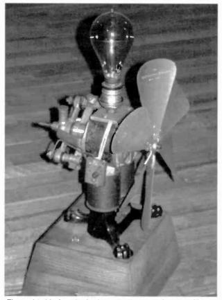
Figure 14. My favorite in the collection, the Curtis & Crocker brass-bladed fan. The light bulb is switched in series with the fan motor for low speed.
