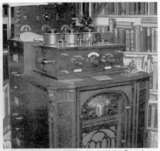
Figure 2. A tuner patterned after the Marconi Multiple Tuner slts atop an Atwater Kent Model 812 console. In the rear is the WE 3B receiver.
