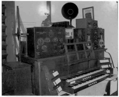
Figure 8. On top of the console of the Aeollan-Skinner organ is the Wireless Specialty Apparatus of 1918, left, and an SE 143, right. The rolls for the player organ go behind the sliding doors above the keyboard. To the left of the console is the DeForest D-10.
