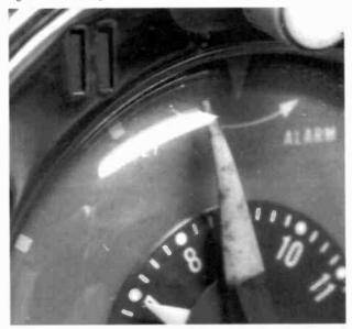
Figure 4. The hands and markings on this clock are a little lumpy and discolored, indicating the likelihood of radium-containing paint.
