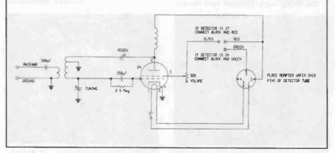
Figure 6. The schematic diagram for the Shorty model adapter.
