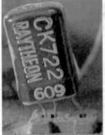
Figure 4. A Raytheon CK722 transistor and socket.
