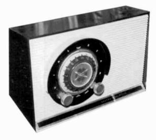
Figure 1. A GE 5-tube AC/DC radio, model unknown, in a two-piece, brown and cream case.
