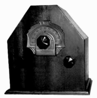
Figure 2. The All-Aire model shortwave adapter uses the same cabinet style as the Shorty, but has a different escutcheon and hexagonal-shaped knobs.
