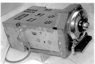
Figure 2. A side view of the car radio. The vibrator and power transformer are located at the rear of the radio.
