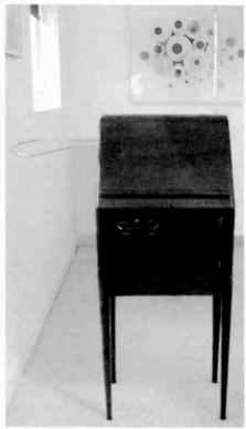
Figure 1. Mark McKeown's restored RCA Theremin. The pitch antenna is on the top and the volume antenna is on the side.
