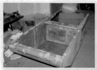
Figure 20. Patches of wet paper towel secured with mylar tape help dent removal.
