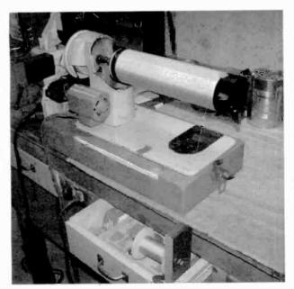
Figure 10. The "Singer" coll-winding lathe. In the lower center of the photograph, note the spool of wire which is being wound onto the right end of the pitch coil on the lathe.
