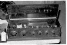
An 8-tube Master superhet complete with tubes. The IF transformers are housed in the wooden enclosure at the rear of the set's cabinet. This set may have been manufactured by the Chicago Radio Labs. It sold for \$400.
