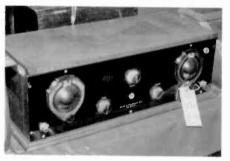
A Smith & Nordstrom 5-tube TRF battery set in a wooden cabinet with an inlaid top cover. The set uses an unusual triple-gang tuning capacitor.
