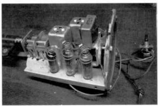
Figure 4. A view of the 5-tube AC/DC chassis.
