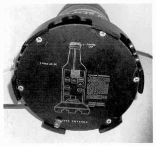
Figure 6. The bottom cover provides a tube layout and operating instructions. An external antenna may be connected to the Fahnestock clip, which can be seen on the lower left of the base.
