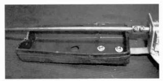
Figure 5. The loop antenna is sized to fit in the Pepsi bottle, and one end is notched to provide clearance for the tuning shaft.
