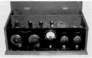
Figure 4. This Hallock and Watson 8-tube superhet used Type UV-199 tubes and a meter to monitor filament voltage.
