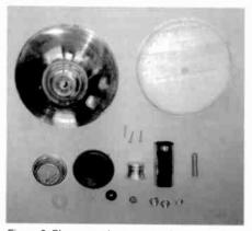
Figure 2. Shown are the parts required to construct the universal base and driver unit. Clockwise from the top: a holder for glass shades, a wooden lamp base, a threaded pipe nipple, a chrome-plated sink drain pipe, and a lamp candle cup along with the Screws, nuts and washers. Two examples of a driver are shown below the shade holder.
