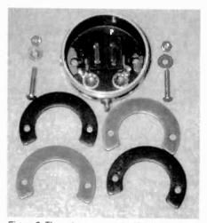
Figure 3. The extra magnets and hardware needed to modify the Federal earphone.
