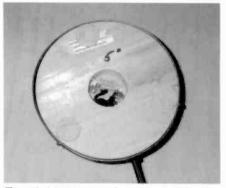
Figure 9. A bottom view of the base with the wooden lamp base, driver, and speaker cable in place.
