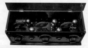
Figure 7. A peek inside the 1925 Model TR-5 shows the set's construction and five Type 01-A tubes.
