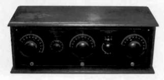
Figure 8. The 1926 version of the Model TR-5 uses four Type 01-A tubes and one Type UX-112.
