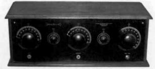
Figure 6. A front view of the 1925 "Halowat" Model TR-5, a TRF 3dialer, which used five Type 01-A tubes.
