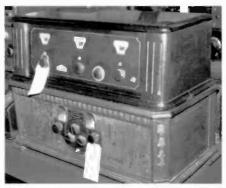
An Amrad Model S522, a 5-tube Neutrodyne, sits atop a Silver-Marshall battery-operated Improved Shielded Lab model.
