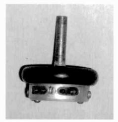
Figure 5. The threaded nipple glued to the cap of the earphone.
