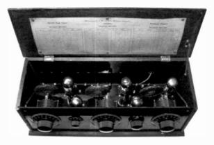
Figure 9. The 1926 Model TR-5 with lid open showing the right-hand selector switch and the instruction sheet under the lid.
