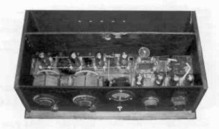
Figure 5. This top view of the 8-tube superhet shows the component layout and bus bar wiring.
