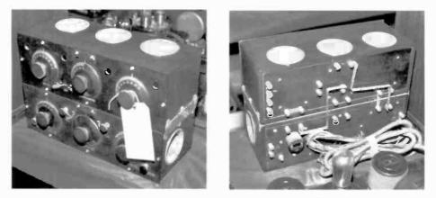
An Amrad combo in very good condition: a Model 3500-1 receiver and a Model 3475 amplifier. With tubes, this pair sold for \$450. The rear view on the right shows the factory flat wiring and the transformer (lower left,) both of which are often missing from these sets.
