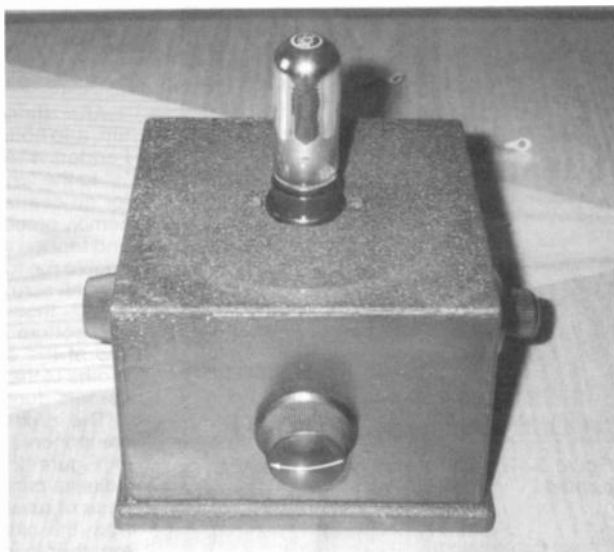
Figure 7. The finished Pseudo Pup with its UV-199 tube in place.
