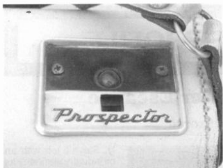
Figure 3. This close-up shows the Geiger counter's neon lamp indicator at the top and the push button below.
