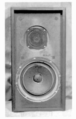
The Model Twenty acoustic suspension speaker with the grille removed. Shown are the f0" woofer and the 134" diameter tweeter cone in a 4½" square basket and black mesh grille cover.
