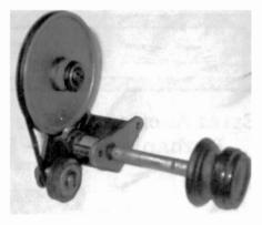
Figure 3. The 2-speed tuning mechanism used in the Model 447.
