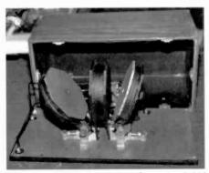
An interior view of the Wireless Speciality IP-503 long wave loading coil.
