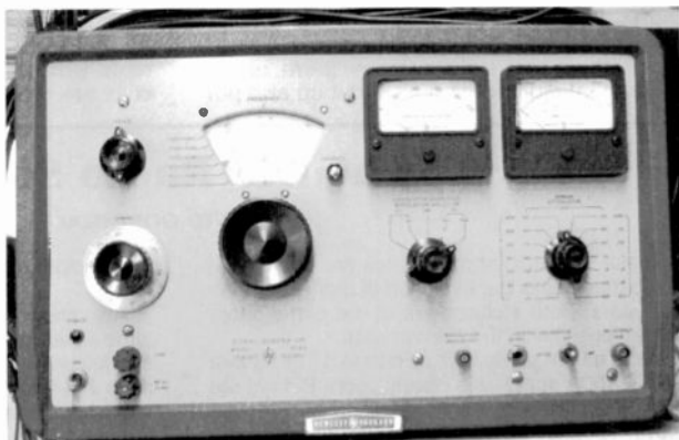
My HP 606A. The meters read "percent modulation" and "output." The unit has an oversized tuning dial and an easy-to-read dial scale.
