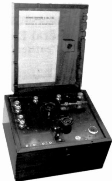
SIEMENS BROS. Type C.V. TUBE/CRYSTAL RECEIVER – Siemens Bros. Co., Ltd., (London) manufactured this one-tube, crystal receiver in 1922. It uses an early V24 tube. The right side of the box can be pulled out in order to give access to the vacuum tube. ( Jim Taylor – Bournemouth, UK )
