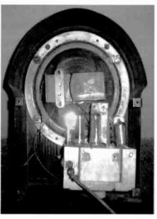
Figure 11. This rear view shows the finished project with the chassis and speaker mounted in the cabinet.
