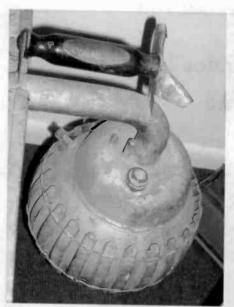
Figure 3. A close-up of the Icyball's pressurized vessel, or "hot ball," that was heated by a flame.
