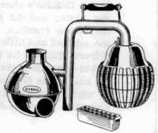
Figure 6. A rendering of the lcyball unit, including the ice cube tray that can be inserted in the "freezing tube," the circular opening at the base of the cold ball.
