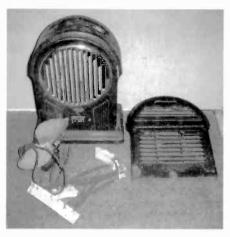
Figure 3. The Sunbeam heater after disassembly. Shown are the metal cabinet, rear panel, fan, and heating elements.
