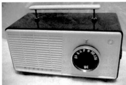
Figure 7. The 9-inch wide Monarch RE 760 has 6 transistors and uses 4 C cells.
