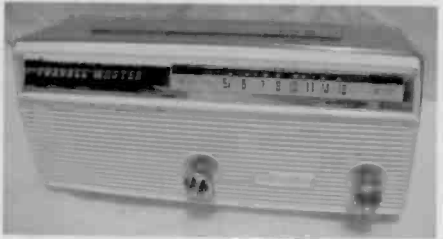
Figure 4. The 10-inch wide Channel Master 6505 has 5 transistors and uses 4 C cells.
