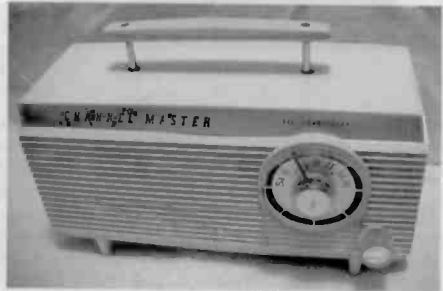
Figure 3. The 6-transistor Channel Master 6500 is 10 inches wide and uses 4 C cells.
