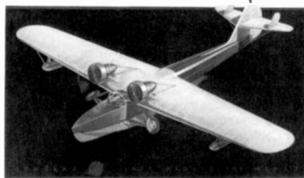
Figure 2. The Douglas "Dolphin" amphibian was the type of personal airplane Crosley preferred. Note that this particular version is without the short stabilizer wing between the engines. Some of the "Dolphins" did away with the triple tail rudders.
