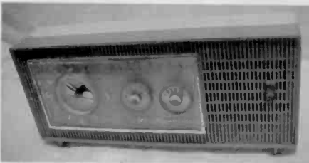
Figure 1. The 1958 Zenith Royal 850, a 7-transistor set with vernier tuning, uses a D cell for the clock and 4 AA cells for the radio.
