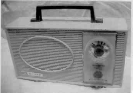
Figure 5. The 10-inch wide Sharp 6H105 has 6 transistors and uses 4 D cells.
