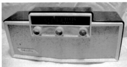
Figure 6. The 15-inch wide, 6-transistor Silvertone 9014 uses 6 D cells and has twin speakers.
