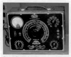
Figure 8. The first Solar Exam-eter, the Model CE "Capacitor Analyzer," used the term "Exam-eter" in the user's manual, but it did not appear on the panel. It was the first Solar analyzer to use a meter rather than an eye tube.
