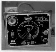
Figure 6. The Solar Model BQC is similar to the QCA but is housed in a smaller cabinet. Also, push buttons are used for the Short Test while the QCA uses slide switches.
