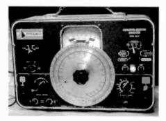
Figure 11. This Pyramid Model CRA-2 Capacitor-Resistor Analyzer is an attractive, well built, and easy-to-use tester. It does it all — it has a quickcheck feature, and it measures resistance and capacitance, leakage, power factor and insulation resistance.
