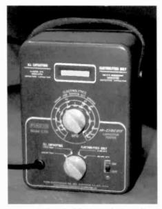
Figure 12. This PACO Model C-25 "In-Circuit Capacitor Tester," uses a modern Type EM84 tube as an indicator. It sold for \$19.95 as a kit or factory wired for \$29.95.
