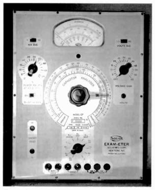
Figure 9. A repackaged Exam-eter, the Model CF, was housed in a larger cabinet with a bigger meter and more modern styling.
