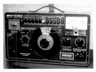
Figure 14. This Sprague Model TO-6 "Sprague Tel-Ohmike" capacitor analyzer uses push buttons to select capacitance scales and test voltages. The analyzer is easy to use. I use it to reform electrolytic capacitors.
