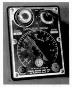
Figure 13. A Cornell-Dubilier Model BN "Capacitor Bridge." This compact tester uses an eye tube as an indicator and measures capacitance values from 10 pF to 50 mF.
