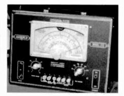
Figure 10. This Jackson Model 112 Condenser Tester uses push buttons and is simple to operate.
