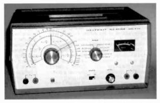
Figure 15. Just one of the many Heathkit capacitor testers and capacitor substitution boxes sold in kit form, this RLC Bridge, Model IB-5821 is a battery-operated, solid-state instrument.
