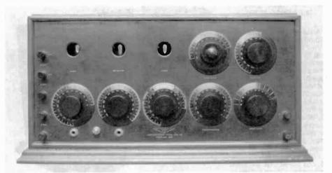
Figure 10. A front view of the Northwestern Model SR-21, a 3-tube regenerative receiver. Peepholes are provided to view the tube filament, and large calibrated knobs are used on the filament rheostats. Battery connections are on the left, and the antennas and ground binding posts are on the right side of the panel.
