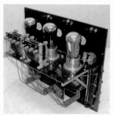
Figure 9. An inside view of the SR-2's chassis shows its components, including the open frame Acme interstage and audio transformers. The unit's on-off switch is located at the far right.
