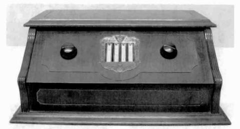
Figure 15. A front view of the 7-tube Model 77 radio. Tuning is accomplished by the four thumbwheel knobs.
