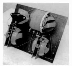
Flgure 6. An interior view of the Type SR-1 showing two variometers at the bottom of the panel and the primary circuit's tuning capacitor and variable inductor at the top. The inductor is tapped, and tap selection is accomplished by the 12-position switch.
