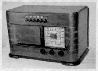
This Philco Model 41-225 is a 6-tube, AC/DC radio that tunes from 550 kHz to 3.3 MHz in two ranges. It features push-button tuning on the BC band.
