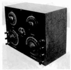
Figure 4. An oblique view of the Type SR-1 regenerative receiver, which is actually a tuner only. The SR-1 uses a Type SR-8 variocoupler and two Type SR-7 variometers.
