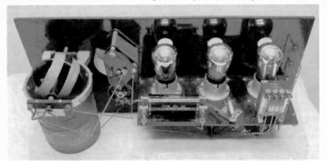
Figure 11. An interior view of the SR-21 shows the tldy layout of its components and the bus-bar wiring.
