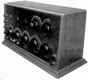
Figure 14. An oblique view of the Northwestern Model SR-21, a 3-tube regenerative receiver. Peepholes are provided to view the tube filament, and large calibrated knobs are used on the filament rheostats. Battery connections are on the left, and the antennas and ground binding posts are on the right side of the panel.
