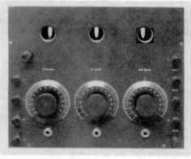
Figure 7. The Type SR-2 detector and 2-stage amplifier is housed in a cabinet 10½" x 12¾" x 6". Peepholes are provided to view the tube filaments. Note the elaborate rheostat knobs.
