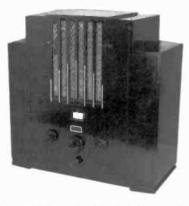
G.E.C. "UNIVERSAL MAINS THREE" RADIO — This is a 3-tube, Bakelite, TRF radio, manufactured in 1934 by the General Electric Company, Ltd., not to be confused with GE, U.S.A. It has a brown Bakelite cabinet measuring 13½" x 13½" x 6½". (Jim Taylor – Bournemouth, UK)
