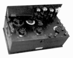
R.I. MODEL V4A – This is a 4-tube radio manufactured in 1922 by Radio Instruments, Ltd., an early quality radio maker. It has an ebonite control panel, a lift-up lid, and a mahogany cabinet. (Jim Taylor – Bournemouth, UK)
