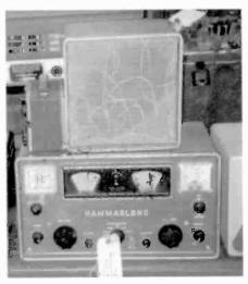
This Hammarlund Model HQ-110 is a 12-tube receiver that tunes seven Ham bands from 160 to 6 meters. In good condition, it sold for \$120. This set has a matching speaker but no clock.
