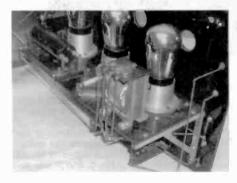
Figure 12. This close-up of the SR-21 chassis shows some of its components, including the interstage audio transformer and a Federal coil.
