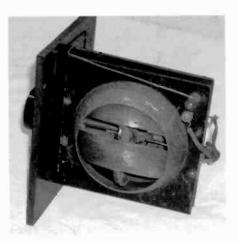
Figure 3. An interior view of the Type SR-23 variometer.
