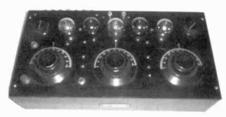
PANDORA, MODEL UNKNOWN – This 5-tube TRF battery radio was made by John Lurie, Jr., of New York, even though it was found in Australia. The serial number is left blank on its oval nameplate. The cabinet is leatherette-covered wood and stands only 5½" high. The battery terminals are mounted on the rear of the cabinet. Is anyone familiar with this receiver or its manufacturer? (Richard Begbie – Bungendore, Australia)
