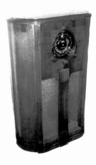
ZENITH MODEL 9S263 – Housed in an unusual oval-shaped cabinet, this 1938 console uses a 9-tube shutter dial chassis with a tuning eye. The tuning range is 500 kHz to 18 MHz. (Tom Ackerman – Germantown, IL)
