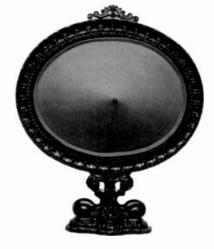
SPLITDORF CONETONE – This elliptical paper cone was manufactured in 1927 by the Splitdorf Radio Corporation of Newark, New Jersey. It was offered as a companion speaker to the Splitdorf Abbey radio. It has a wooden back and sits atop a papier-mâché stand that swivels. It stands 26" tall and 22" wide. (Ross Mason – Mason City, IA)
