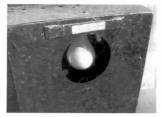
Figure 3. Back of the display sign with the access panel removed for replacing the bulb.
