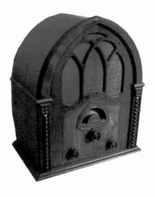
ATWATER KENT MODEL 82 – This Gothic cathedral was manufactured in 1931. It is a 7-tube, ACoperated, superheterodyne radio and is one of the many 80 and 90 Series radios Atwater Kent manufactured in 1931 and 1932. The Model 82-D was a DC version, while the Model 82-Q was a battery (or farm) receiver. (Dave Crocker – Mashpee, MA)
