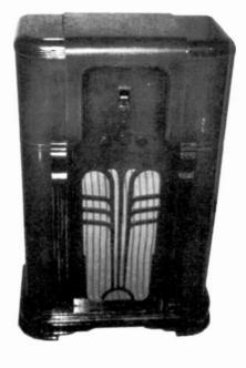
PATTERSON, MODEL UNKNOWN – This 17-tube, 4-band console, was manufactured by the Patterson Electric Co., ca. 1934. Patterson was more widely known for military and Amateur receivers. The set was advertised in our local newspaper as a "1920s, floor model transistor radio in very good condition." I was glad to releve the owner of what he called, "this old thing." (Carl D. Sutton – Ironton, OH)
