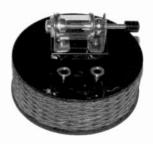
MOTALAREN – This crystal set was made in Sweden. It is an outstanding design built in a coil and using a plug in-detector, which was also made by a Swedish company called EKA. (Erwin Macho - Vienna, Austria)
