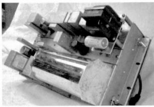
Figure 3. This rear view of the unit shows the added power supply at the upper right.
