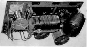
This Type SE-1420C Medium Wave Receiver was manufactured for the Navy by American Radio & Research Corp. (AMRAD) in 1920. It has a coverage of 250 to 7,500 meters and sold for \$7,000.
