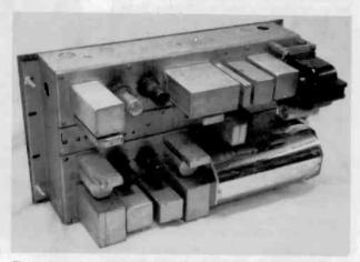
Figure 2. A rear view of the Frequency Standard shows the neatly arranged components and tubes. The crystal oven is the shiny chrome-plated device in the lower right.
