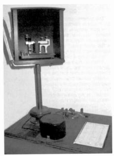
Figure 2. Telegraph sounder and resonator.
