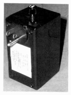
Figure 2. A rear view of the Soft-Starter, Model AB1M, showing a 3-prong AC plug. Mounted on top is a fuse holder containing a 1.25A fuse.
