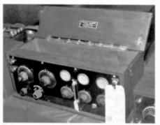
This 3-tube Trego radio, manufactured in Kansas City, Missouri, sold for \$145. The control at the lower left is an add-on.
