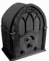
ATWATER KENT MODEL 82 – This Gothic cathedral is a 7-tube superheterodyne radio, one of many 80 and 90 series radios manufactured by Atwater Kent in 1931 and 1932. The Model 82-D was a DC version while the Model 82-Q was a battery (or farm) receiver. (Dave Crocker – Mashpee, MA)
