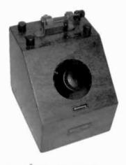
KAPSCH U. SÖHNE CRYSTAL SET—I looked for about 25 years for this Austrian novelty from which only one piece is known. Finally, I bought it from a collector who sold his complete collection. It was built in 1924 and uses condensator tuning. The original detector had been lost, but I found the right parts and completed this wonderful set. Now it is the "Star" in my collection. (Erwin Macho – Vienna, Austria)
