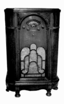
ATWATER KENT MODEL 310 – This 6-legged console was manufactured in 1933. It operates using the following tube types: (3) 58, (3) 56, (1) 80 rectifier, and (1) 56 oscillator. It tunes the broadcast band and one shortwave band. Below the main dias a smaller dial for fine tuning. (Ross Mason – Mason City, IA)
