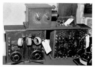
An unidentified loose coupler with a crystal detector sits atop a 2-unit home-brew radio that sold for \$1,700. The home-brew set consists of a 1-tube tuner with honeycomb coils and a 3-tube amplifier.
