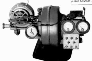
MORSE CHAPMAN WAVE GENERATOR – This unit was manufactured in Boston, Mass., by the Morse Chapman Company. It has two meters: a 0-200 voltmeter on the left and a 0-50 milliammeter on the right. On the far left is a sine-wavemeter indicator numbered from 1 to 10. A GE 110-volt motor, Type 5A, with a patent date of January 1905, drives the unit. (Frank Moore – Billings, MT)
