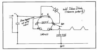
Figure 1. Wiring sketch of a typical halfwave rectification circuit where the added diode is connected between cathode and plate terminals of the rectifier tube socket. Since the diode replaces the function of the rectifier, the rectifier tube must be removed.
