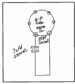
Figure 2. Wiring sketch for the added 7 microfarad capacitor on the 6-pin tube base.
