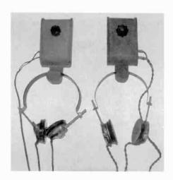
BLAUPUNKT CRYSTAL SET – Made in Germany, this 1945/46 crystal set is very well known. It was built in two different condenser tuning versions and is designed for wall hanging and for mounting headsets. (Erwin Macho – Vienna, Austria)
