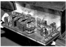
An interior view of the mystery radio. The modified 4D chassis is on the left, and an amplifier with one of the Western Electric tubes is on the right.
