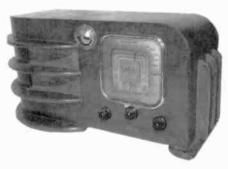
GENERAL TELEVISION, EMERALD MODEL — This all-wood cabinet radio, ca. 1939-1940, was built by the General Radio and Television Corp. of Chicago. It has a 6-tube circuit with a bias cell. The tuning eye tube is a Type 6G5. It tunes both the broadcast and shortwave bands. A smaller version was named the "Baby Emerald." (Jim Knapp — Phoenix, MD)
