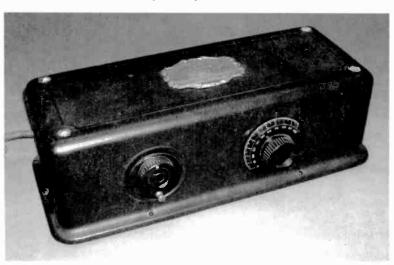
The Atwater Kent Model 35, a 6-tube TRF, was introduced in 1926, and is commonly referred to as the "bathtub set."
