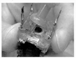
Figure 2. After removing the IF transformer from its can, a pushpin was used to lift one of the metal tabs that make contact with the mica capacitors.
