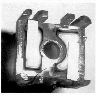
Figure 1. This view of a typical "new design" IF transformer shows the silver migration pattern on its mica capacitors. The migration is seen as the dark, shaded outline around each of the capacitors.
