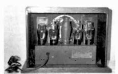
Figure 2. A rear view of the Kadette 86X showing its five tubes.
