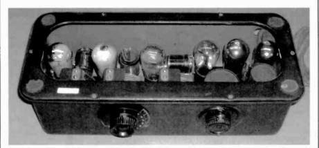
An underside view of the Atwater Kent Model 35 showing the upside-down chassis and tubes.
