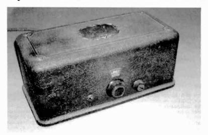
The Day-Fan 6 Jr., a 6-tube TRF introduced in 1927, is similar in style to the Atwater Kent 35 introduced the previous year.
