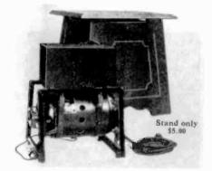
Figure 5. The motor generator and power filter shown in front is for use in a basement, or it can be concealed in the optional "tabouret" in the rear.
