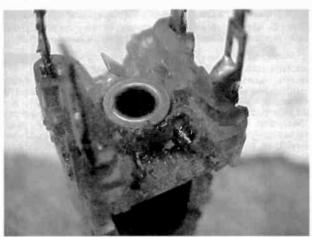
Figure 3. This view shows one of the tabs lifted (rear) and one section of the mica capacitor removed (foreground).
