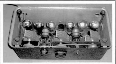
An underside view of the Day-Fan 6 Jr., showing the upside-down chassis and tubes, similar to those of the Atwater Kent Model 35.
