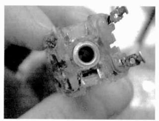
Figure 4. In this view, both of the mica capacitor sections have been removed.
