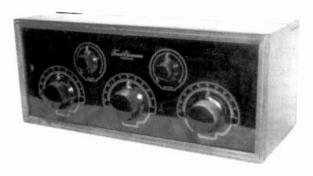
FREED-EISEMANN MODEL 10 – This 5-tube battery receiver was manufactured in 1926 in New York City by the Freed-Eisemann Radio Corporation. It uses Type 201A tubes in its Neutrodyne circuit. (Wally Worth – Wollaston, MA)
