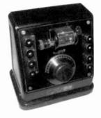
ISARIA TYPE D CRYSTAL SET— This rare crystal set was manufactured by Isaria Zählerwerke in 1924/25. It is a German set with variometer tuning and a black metal case. The plug-in crystal detector is called "Red Star," a very expensive component. (Erwin Macho – Vienna, Austria)
