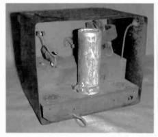
Figure 2. An "as-found" photograph of the Crosley 2C1. The mechanical connection between the magnetic driver and the front-panel diaphragm can be seen at the center of the figure.
