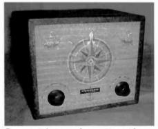
Figure 1. This 2-tube Crosley Model 2C1, ca. 1934, has some unique features, including the cardboard panel/speaker diaphragm.
