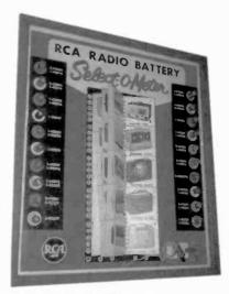
RCA "SELECT-O-METER" – This RCA battery selector for portables would be found at a repair counter for public use. First, one would locate the radio of interest from the splral-bound center pamphlet, and then, using the wire, plug into the jack indicated. One of the lights on either side would then Indicate what battery combination was required. A "D" battery, placed in the space at lower right, powered it all. (Paul Check – Lodi. NJ)
