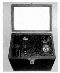
Figure 1. T&H Manufacturing's Model 60 Analyzer is an example of an early capacitor test set.
