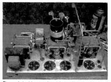
Figure 6. In this rear view, disassembly of the transmitter is underway. The front panel has been removed. The modulation transformer is located in the lower left corner and the microphone transformer is in the upper left next to the variable capacitor.
