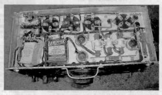
Figure 4. The underside of the chassis was relatively untouched with only some minor wiring changes and the replacement of a capacitor.
