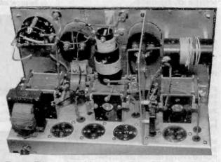
Figure 3. This rear view of the transmitter shows its condition prior to restoration. Numerous modifications had been made to the set by a previous owner.
