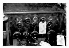
This Airway Type G, circa 1923, with a rheostat control for each tube filament brought \$2,000 in the auction.
