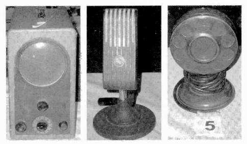
Left to right: this heavy Teletone TV must be a portable – it has a handle! Center is another contest entry in the microphone category, an RCA ribbon microphone. Right is an early carbon microphone.
