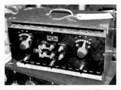
A Lane SYD Alkaline storage battery. This wet-cell B battery has selectable voltage outputs and a changeover switch to allow charging.
