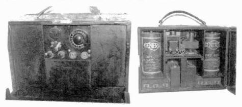
**KODEL MODEL P-12** – This 2-tube leatherette "Fabricoid" portable was produced in 1924 by the Kodel Manufacturing Co. of Cincinnati, Ohio. It was the next step up from Kodel's Model P-11 1-tube portable, so small it was called the "Camera Radio." Note that the tapped coil fits around the Type 199 tube in the photo at the right. (*Wally Worth – Wollaston, MA*)
