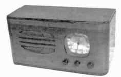
KADETTE MODEL 1019 – This shortwave and broadcast band radio was advertised as having 10 tubes, although two are ballasts and two are redundant. ((Ray Chase – Plainfield, NJ
