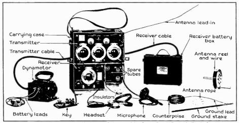
Figure 1. The transmitter described in this article is part of the Coast Guard Portable Radio Station shown here with its accessories.
