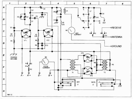
Figure 13. A schematic diagram prepared by the author as part of the restoration work. The associated parts list is shown in Table I.
