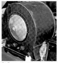
This Thompson Minuet, ca. 1925, uses a unique tuning arrangement that is positioned around the edge of the speaker. A 5-tube battery set, it sold for \$7,000.
