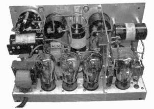
Figure 11. A rear view of the restored transmitter with all components and tubes in place.
