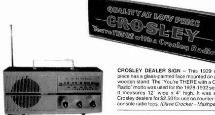
RIVIERA HI-FI DELUXE - This 6-transistor AM receiver was manufactured in Japan by the Nissho Electronics Corp. I purchased this radio in 1965 for \$25 in Santo Domingo while in the army. It has a wooden cabinet and a plastic front face, and uses four D batteries. (Loren P Ashworth - New Paris, OH)
