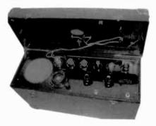
GLED TYPE P-9 - Manufactured by the Gled Radio Co. of Philadelphia, this 6-tube portable uses six Type 199 tubes. The speaker is panel-mounted and is housed in a leatherette-covered case. The loop antenna is mounted in the lid of the case and is removable. (Wally Worth - Wollaston, MA)
