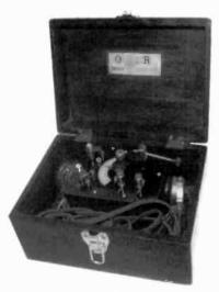
ORATOR CRYSTAL RADIO – This "midget radio" crystal set was manufactured by the Orator Mfg. Co. of New York. It operates using a galena/catwhisker detector. Included In Its wooden case is a pair of headphones. It sold for \$15 in 1926 (Wally Worth – Wollaston, MA)
