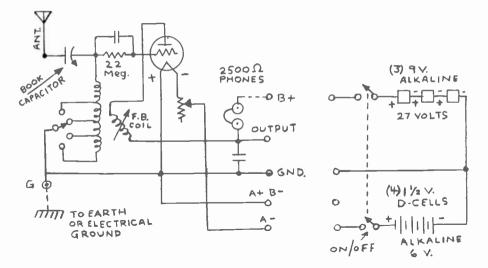
Figure 3. The Crosley Model 50 circuit diagram at the left, and the home-built battery box circuit at the right.
