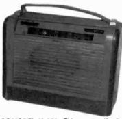
PHILCO MODEL 46-350 – This wood and leatherette portable receiver, manufactured in 1946, has a tambour cover that rolls over the dial. It tunes the AM band only, using a 6-tube chassis. The tube complement is the following: (2) 1T4, (1) 1R5, (1) 1U5, (1) 3LF4, and (1) 117Z3. (Clark Trissell – Lincoln, NE)
