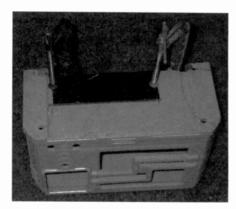
Figure 2. A replacement piece of Bakelite is clamped in place in preparation for gluing.
