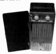
ASTOR MODEL KQ – This is an Australian portable pocket radio of 1947 vintage. It covers the standard AM broadcast band using a miniature 4-tube lineup. The loop antenna is housed in the Bakelite cover which activates an on/off switch when opened. Filament power is supplied by two 1.5V D cells and B+ by a 67.5V battery. What is unusual about this radio is that the tuning dial is marked 1-10 rather than the usual 55-160 designation for the AM broadcast band. (Rich Smardzewski – Bel Air, MD)
