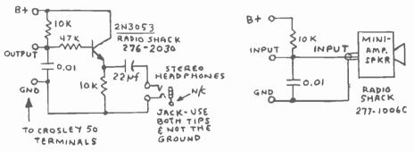
Figure 4. The emitter-follower impedance transformer diagram for low impedance headphones at the left, and an alternative circuit with volume gain at the right.
