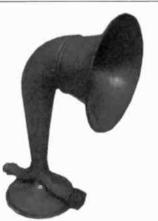
KING AM-PLI-TONE – This unusual horn speaker has no reproducer. It uses a pair of the operator's headphones clamped on the two openings at the bottom. (This horn is missing one of the rubber headphone seals.) The horn is 14½" tall and is made of cast aluminum with a plated tin bell and heavy cast iron base. Imprinted inside the bottom of the base is "King Co., New York." (Dave Crocker – Mashpee, MA)
