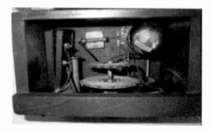
Figure 2. Looking down into the interior of the Crosley Model 50, showing the patented booktype tuning condenser and the operating cam shaft at the left.
