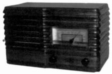
AIR KING MODEL 252 – This stylish receiver of the late 1930s uses the following tubes: (1) Type 6A7, (1) Type 6D6, (1) Type 75, (1) Type 25L6, (1) Type 25Z5, and a ballast tube. (Clark Trissell – Lincoln, NB)
