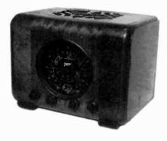
**ZENITH MODEL 6S222** – This set, manufactured in 1937, is one of the many "big black dial" radios of that era. It has a 6-tube chassis, and because of its cube shape, the speaker grille is on the top. It tunes both the broadcast and shortwave bands. (Clark Trissell – Lincoln, NE)
