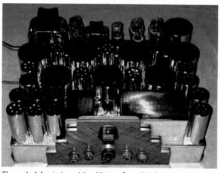
Figure 1. A front view of the 23-tube Scott Full Range High Fidelity receiver.
