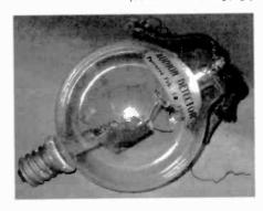
De Forest Wireless Company Single Wing Audion vacuum tube, 1909. This was the first commercial, 3-element vacuum tube placed on the market, and it enabled wireless signals to be amplified for the first time. This tube is complete with good filaments and original label.
