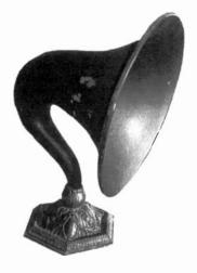
STEWART-WARNER MODEL 400 – This hom speaker was manufactured by the Stewart-Warner Speedometer Co. of Chicago. The 15" diameter fiber bell sits on a heavy cast metal "tulip-styled" base. Its original price was \$25. (Dave Crocker – Mashpee, MA)
