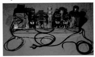
Figure 12. The recording amplifier used in the 48-tube custom receiver.
